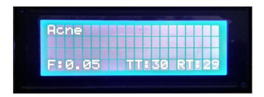
6. Press "START/STOP" button to start the frequencies. Now display shows disease name - "Acne", Initial frequency - "F: 0.05", Total time in minute (T) - "T":30", Remaining time in minute (R) - "R":29.At the same time ON/OFF LED will blink. The frequency will be changed automatically after 3 minutes. When we press "START/STOP" button again the operation will be stopped and device will stop to generate frequencies. At the same time ON/OFF LED will OFF.
